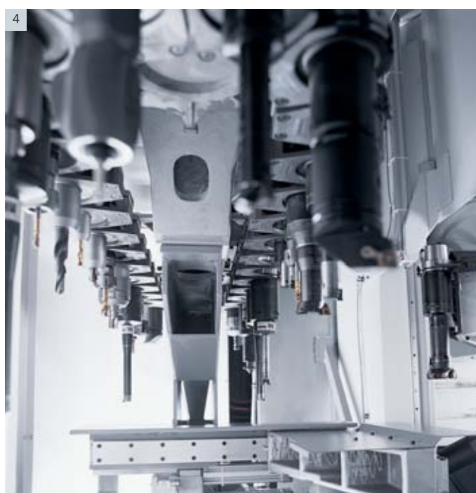
1|–2| Vertical chain magazine for up to 120 tools (SK40 / HSK-A63) and 650 mm max. tool length |3| Fast cam-controlled double gripper for short chip-to-chip times (3.7 sec. for HSK-A63) |4| Horizontal chain magazine for up to 120 tools with SK50 / HSK-A100 (not with DMU 160 P / FD)
