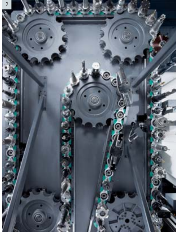
11) Faster and more space-saving pallet changer for set-up of work pieces up to 3,000 kg parallel to production time 12) Vertical chain magazine with a fast curve-controlled double gripper for short chip-to-chip-times of up to 3.7 seconds
