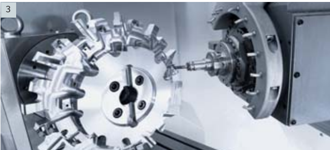
11–21 NC-controlled swivel milling head as B-axis for simultaneous 5-axis milling with high precision by machining at the intersection of multiple axes 131 Dividing device and B-axis as customized solution in toolmaking, for example 141 NC-controlled A-axis – for simultaneous 5-axis milling with negative angles up to -30^\circ
